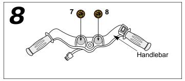
• Apply labels #7 and #8 to the handlebar, as shown.
